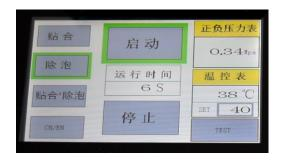
Press the start button , equipment start work , run until the set defoaming time , at this time equipment start for defoaming , to set the defoaming time , equipment began to deflate , pressure to zero , finishing the bubble remover.
