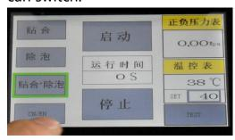
Press TEST twice to set the device parameters.
