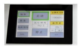
Press the start button , equipment start work , machine start vacuum pumping , run until the set laminating time , pressure gauge go up , at this time equipment start for laminating , to set the laminating time , equipment began to deflate, pressure to zero, finishing laminating.
