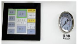
\*Each region is different altitudes , will affect the effect of vacuum , the higher the altitude , negative pressure peak is lower , negative pressure more than -88 for best effect.
