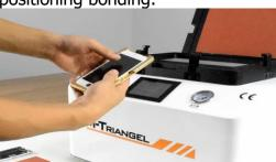
\*Pay attention to the cover plate and LCD , don't squeeze pressure, usually there will be a hollow out after middle at the bottom of the mold, only need the finger on the cover board, again in the middle of the mold at the bottom of the tap the LCD, do the middle stick to so far, this is extremely important!
