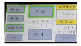
Press the start button , equipment start work , observation pressure gauge , temperature control meter , pressure gauge to zero , after the completion of the laminating , device automatically jumps to the bubble removal pattern , to set the time equipment to deflate , running time to zero , finishing the laminating bubble
